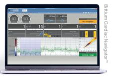
**Bittium Faros™ devices** are delivered with software for changing the measurement settings of the device and to view the recorded ECG data.
